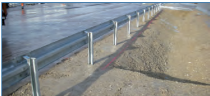
Test set-up EASY-RAIL 2.00 on slope
